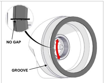
**8. Acetal washer placement** Stretch the split washer gently and fit it into the groove.
