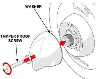
Fit the handle so the arrow shape on top of the handle matches the marking on the faceplate. Keep the washer in the groove of the handle and push the handle into the flange and fasten with supplied tamper proof screw.
